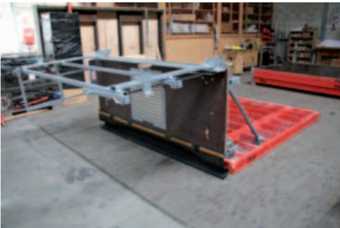
5. Secure diagonal bracing in the panel struts.
