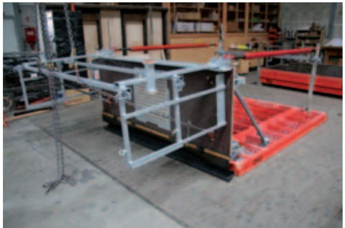
6. Mount push-pull props and horizontal struts.
