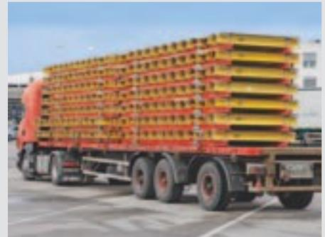
14 VD 250/265 x 600 tables, 223 m<sup>2</sup>, are transportable on one truck.
