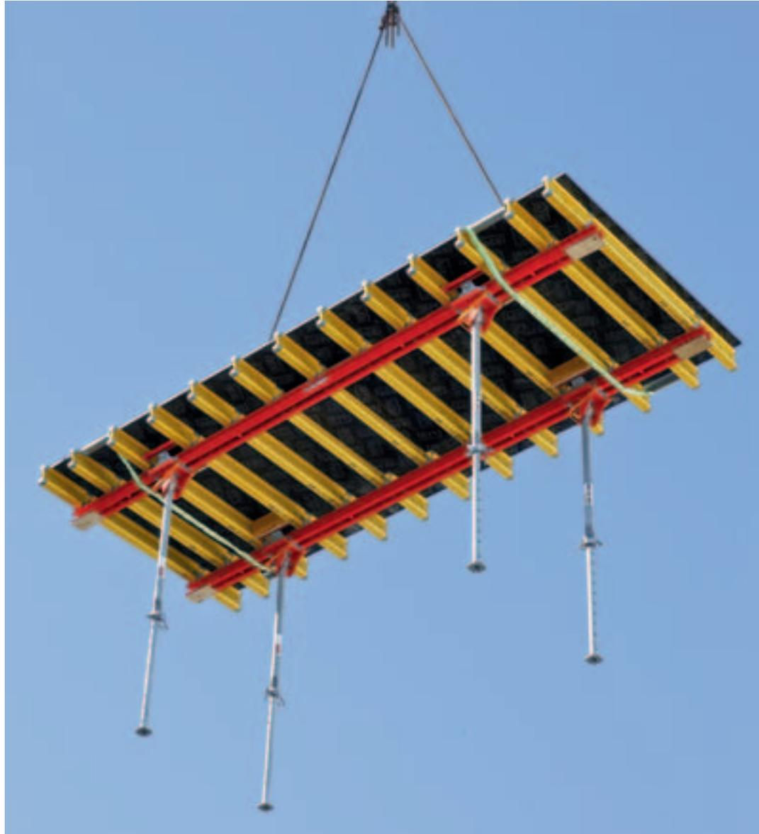
VARIODECK steel waler slab table with dimensions of 2.50/2.65 x 6.00 m requires only 4 slab props. This corresponds to a maximum 4 m<sup>2</sup> of slab per prop.
