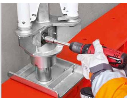
The lowering device has a 10 cm lowering range for easier striking when fully loaded, tiltable on all sides up to 3°.
