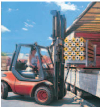
The PERI post pallets are designed for the loading dimensions of a lorry. They can be lifted using the longitudinal as well as end sides.
