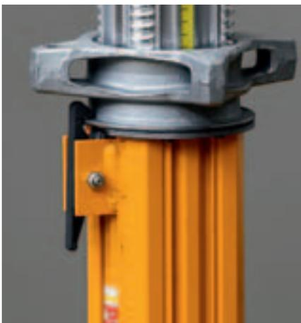
The securing hook prevents the inner tube from slipping out and must be properly engaged for correct transportation procedure.
