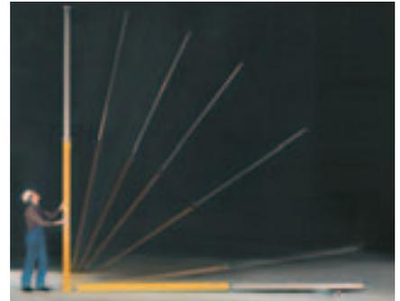
In drop tests on a transversely positioned steel tube, an extended MULTIPROP Prop remains completely undamaged – in contrast to, e.g. tubular steel props.
